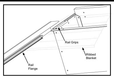
Close the tailgate and pull the <u>rails only</u> toward it leaving approximately 1/8" gap between the end of the rails and the tailgate.
