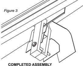
Be sure to hold the rail down and the clamp up while tightening the bolts in the clamps. This will insure a snug fir to the Truck bed. Do Not Over Tighten the Clamps.
