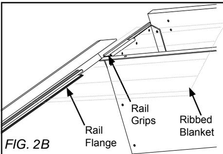
Starting with either rail you will need to hold the rail level and slide the lower rail (**male profile**) into the rail grip (**female profile**) that is bolted to each side of the canister (Fig. 2B). You must hold the ribbed blanket out and level while sliding the rail over it and into the rail grip on the canister. (Fig. 2C) Tilting the rail to get it inserted right then bringing it level works well. (Fig. 2D)
