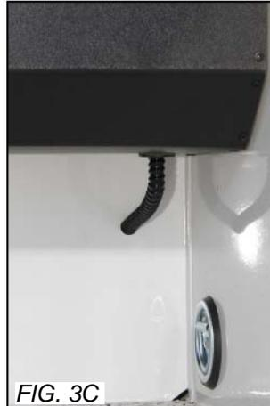
The drain tube should click into place.
