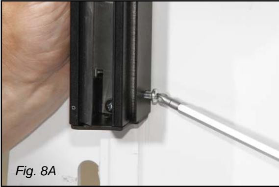
Temporarily remove the end cap screw. (Figure 8A)
