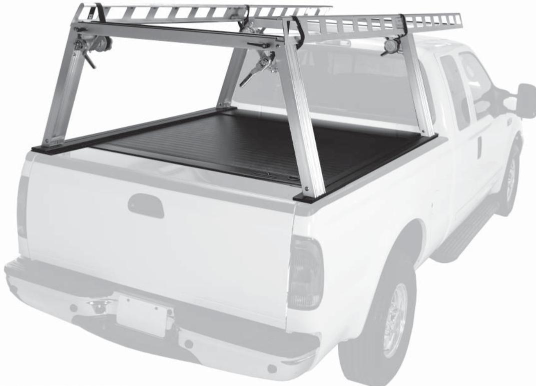
**IMPORTANT!** The Pace Edwards truck bed cover and Explorer Series Rails **MUST** be installed on the truck first before attempting to install this rack system!
